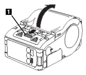
3. Place the label roll in the printer. Make sure it is placed with the leading edge (1) feeding up from the bottom of the roll and not down from the top.
